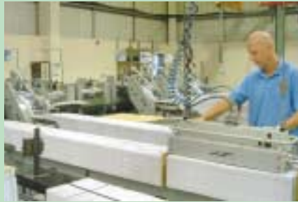
Loading sections onto the perfect binder
